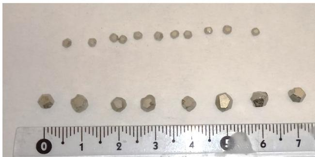
Figure 7.1. Pyrite samples used in the experiments carried out.
