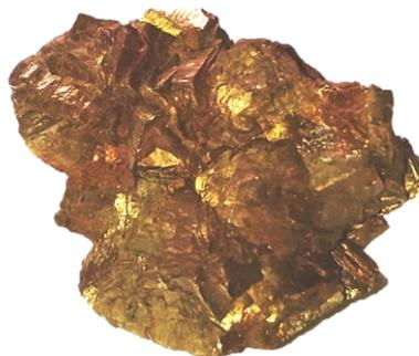
*Figure 2.1. Partially oxidized pyrite sample. The reddish patina in some areas of the surface is a symptom of the formation of iron oxides.*
